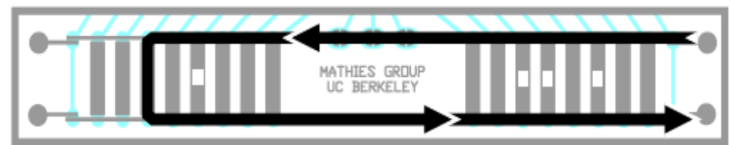
(B) Load input DNA into fluidic loop and chamber
